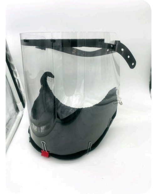
6. Elastic was added and test fits were done with clips.
