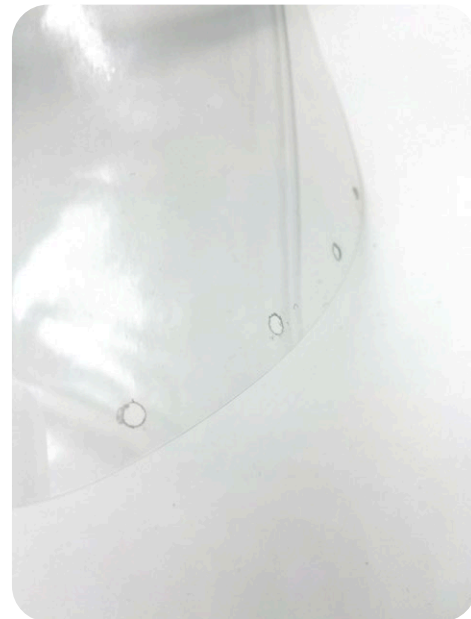
9. Holes were added to the shield for snap placement.
