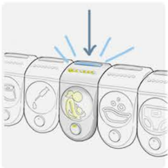
7. Mom can indicate questions by pressing top blue button. Next clinician that enters room is aware.
